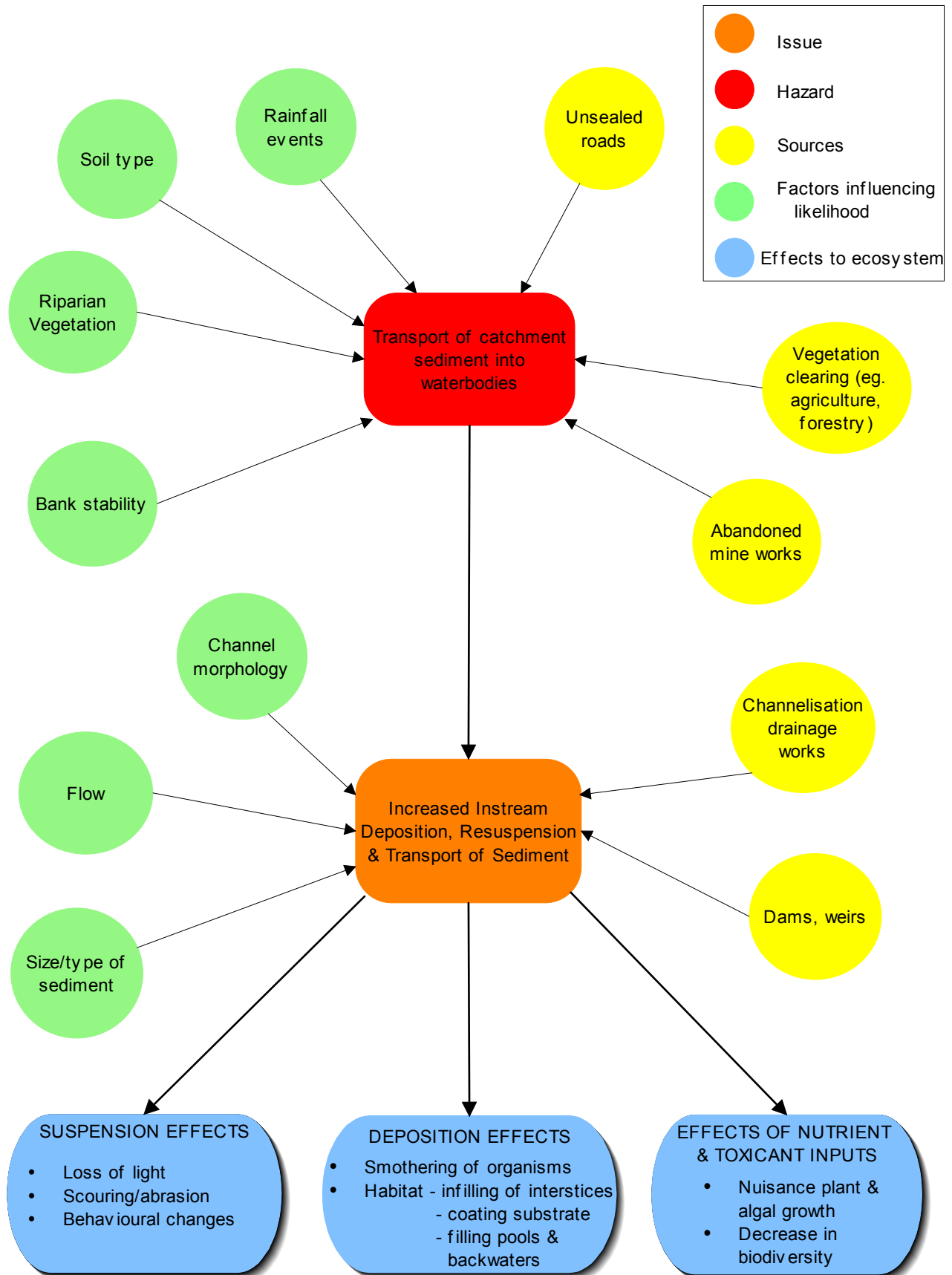
Figure 9: Upper Barwon catchment conceptual model for the issue of excessive sediment inputs
