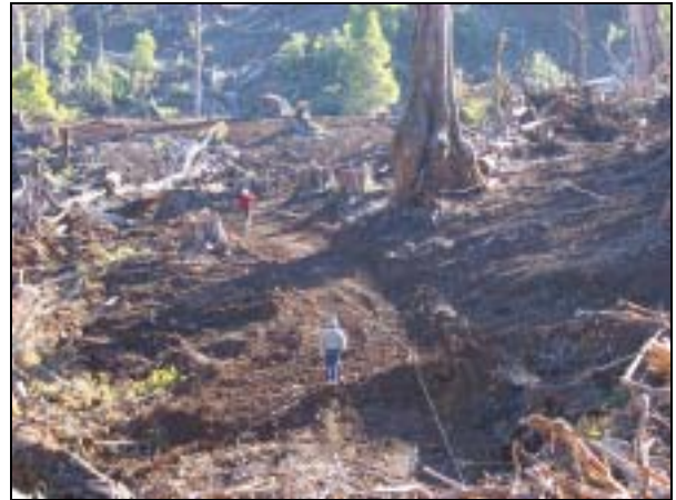
Photo 10. An example of measurement of cross-drain installation distances and slope of snig track.
