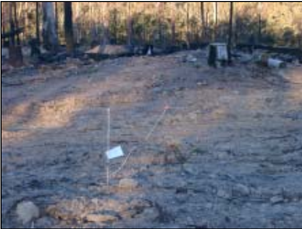
Photo 7. An example of measurement of log landing ripping width and depth.
