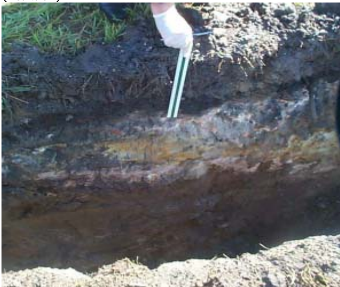
5. Excavation of test pit showing basalt at edge of quarry (10/4/02)
