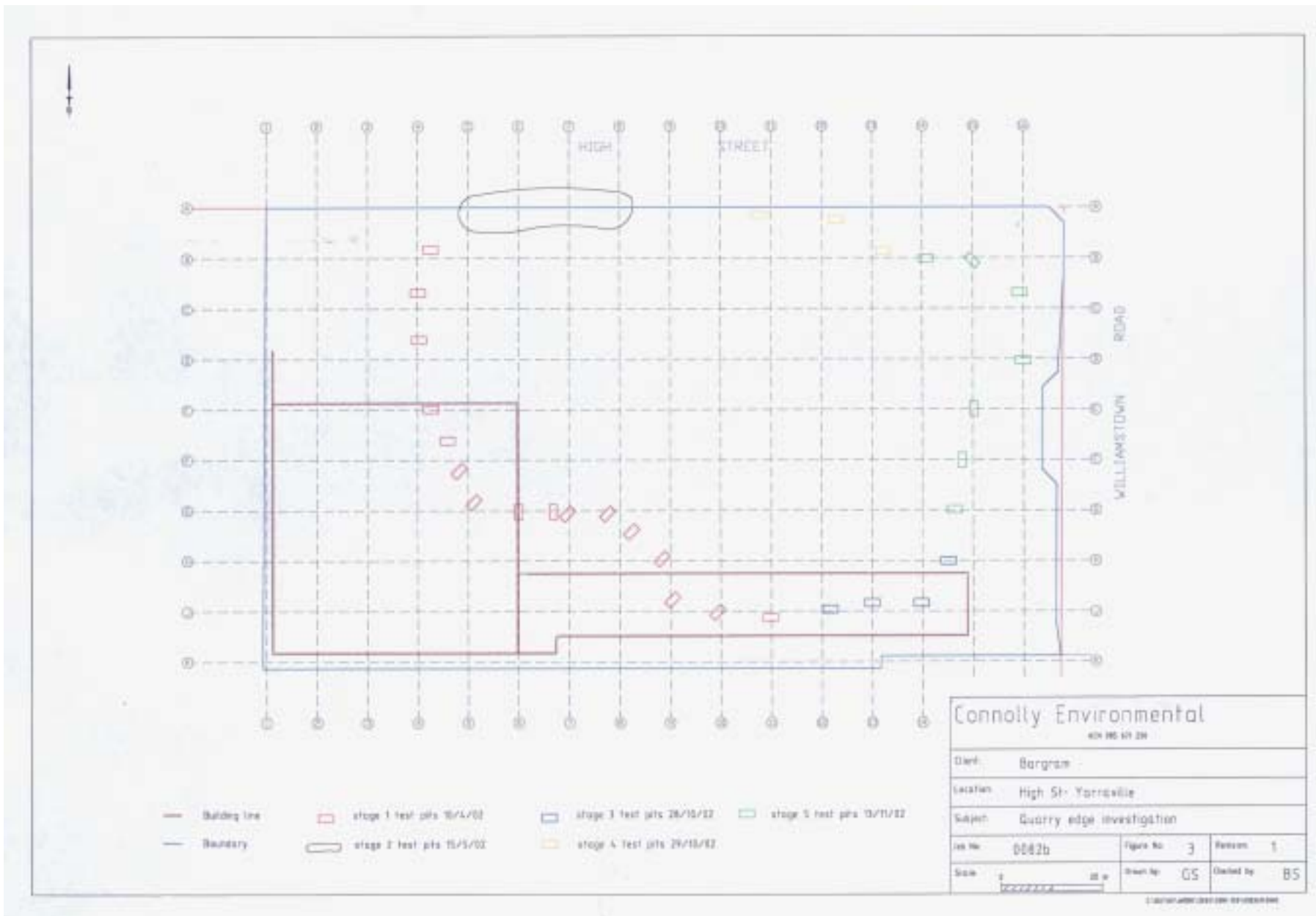
FIGURE 11 TEST PITS TO LOCATE QUARRY EDGE
